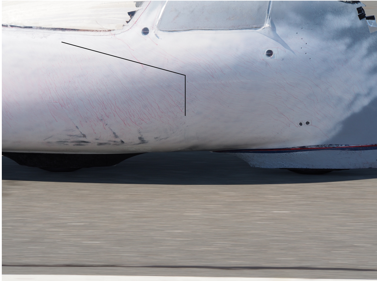
Figure 4.8: Shear fluid testing over Bluenose at U_\infty = 100\text{km/hr} , \rho_\infty = 1.13\text{kg/m}^3 .
