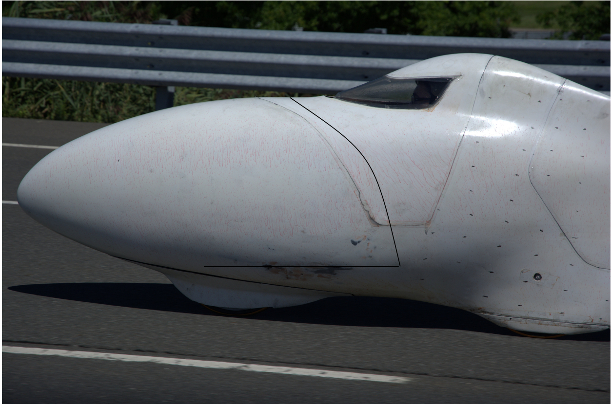
Figure 4.3: Shear fluid visualization on the University of Toronto's HPV Design Team's Vortex at U_\infty = 80\text{km/hr} , \rho = 1.13\text{kg/m}^3 at Ford's Michigan Proving Grounds, Romeo, MI. The shear fluid visualization method is discussed in 4.3.1. The black line indicates the boundary-layer transition line.
